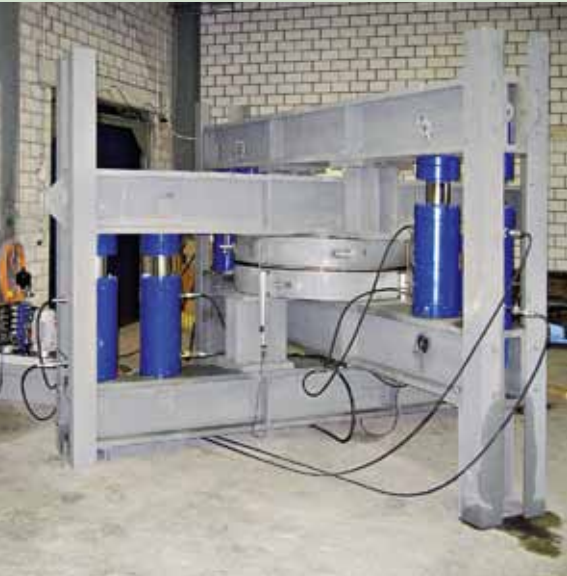
Firm's own joint testing equipment ( Q_{max} = 3000 \text{ kN} )
