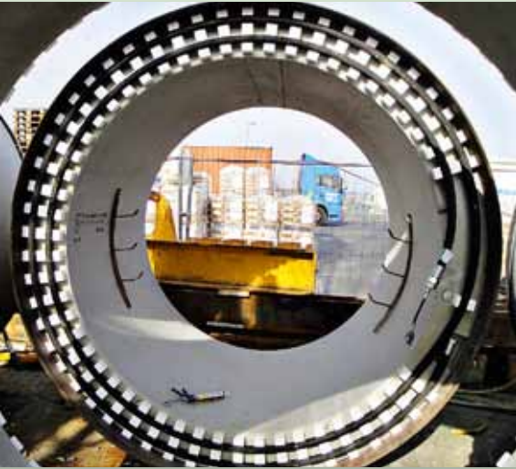
Jacking pipe DN2000, equipped with Hydraulic Joint, ready for installation
