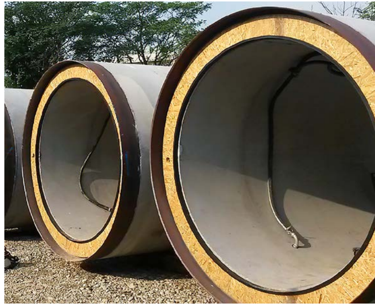
PRESSURE TRANSFER RING (PTR) MADE OF TIMBER
