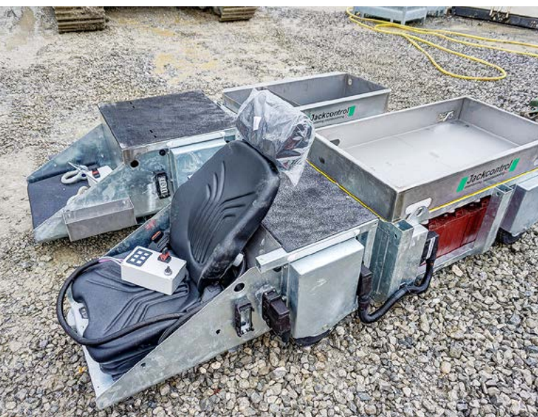
MULTIFUNCTIONAL, SELF-SUFFICIENT TUNNEL VEHICLE CT ROVER, CONSISTING OF TWO COMPONENT VEHICLES
