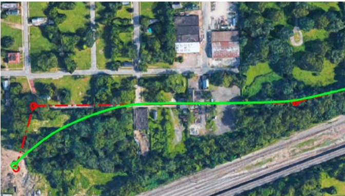
MICROTUNNEL IN CLEVELAND, OH (USA): ALIGNMENT OPTIMISATION WITH HYDRAULIC JOINT
